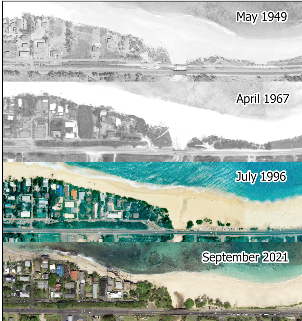
Figure 5. Erosion of Sunset Beach over time. (Source of Images: Climate Resilience Collaborative, 2022b. Figure compiled by Authors.) Though images depicted are taken at different times of the year, and beach widths on the North Shore of O'ahu vary depending on seasonality, there is documentation of chronic erosion occurring in this area (Climate Resilience Collaborative, 2022a).
