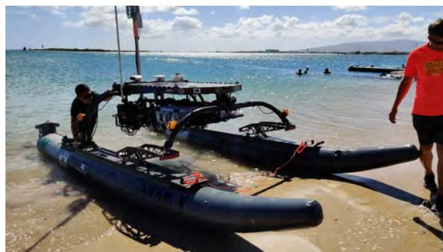
**Photo:** A 16-foot-long unmanned seafaring vessel called the Wave Adaptive Modular Vessel (WAM-V) at Sand Island
