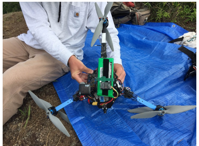
Figures 2 and 3: Flight mission while the flight was underway and the Y-6 rotary UAV being prepped for launch.
