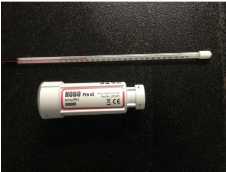
Figure A. Electronic and analog means to monitor temperatures in environmental chambers.
