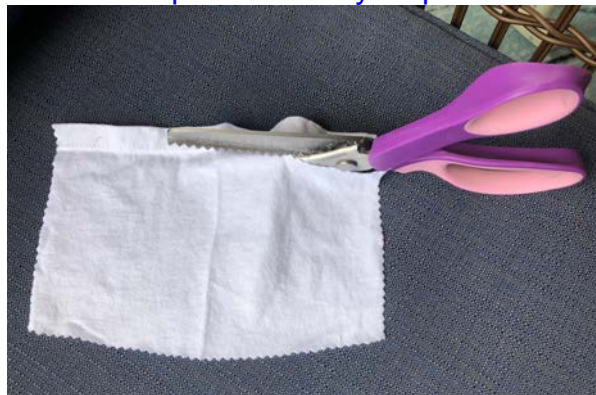
Fig. 5 Pinking shears cut in a zig-zag pattern to stop the edges from fraying. Image courtesy of Karen Duncan.
