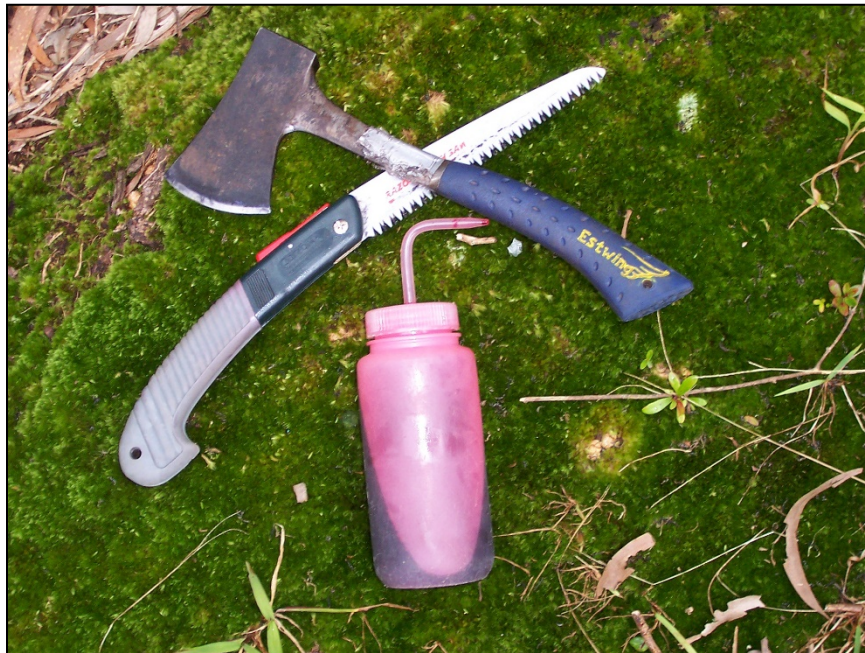
Weed control hand tools including hand pruning saw, hand axe and 500 ml Applicator bottle with 20% Garlon 4 in biodiesel carrier oil
