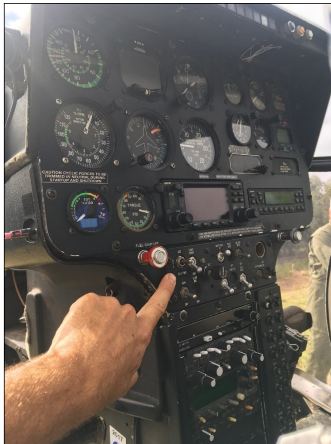
Fuel and Battery shut-off in K&S 1PH
